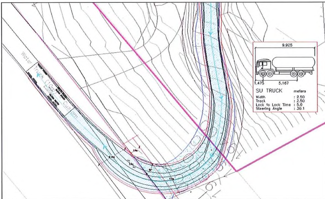
FIGURE 6.1 – 9.9 METRE SINGLE UNIT TRUCK ON-SITE MANOEUVRING
