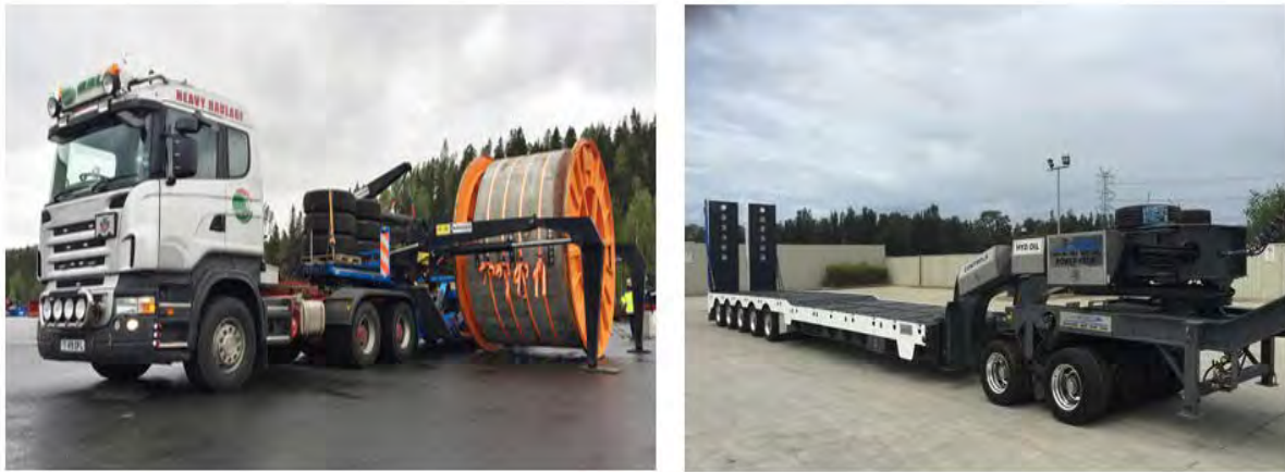
Figure 2-35. Examples of low loader trailers used to transport cable drums (Source: Prysmian)
