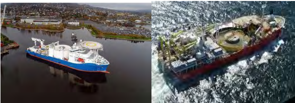
Figure 2-50. Examples of cable lay vessels (Source: Left: NKT, Right: Nexans)
